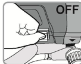
7. Sprayer will start pumping and water or flushing solvent as well as air bubbles will be purged from system. Let fluids discharge from Priming Tube into waste bucket for 30 to 60 seconds then switch Power to OFF
