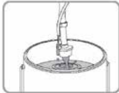
1. Relieve pressure and drain paint from tubes
