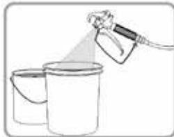
9. Change to waste bucket as paint thins
