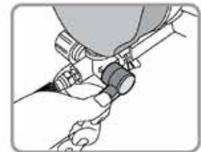
11. Turn Prime/Spray switch to Spray mode and continue to spray into waste bucket
