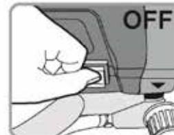
12. Release trigger, turn power OFF and relieve pressure
