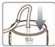
3. Submerge Suction Tube in water or flushing solvent
