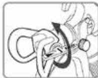
5. Unthread Spray Tip and remove
