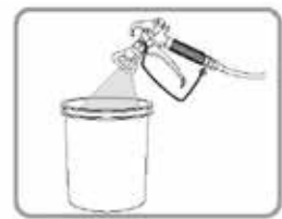
10. Paint should work itself from Suction Tube to Sprayer to Priming Tube until paint discharges from Return Tube. Point gun into waste bucket and pull trigger.
