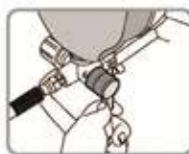
4. Turn Prime/Spray switch to Prime mode
