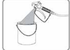
8. Spray paint into paint pail
