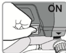
6. Plug in Sprayer and turn power to ON
